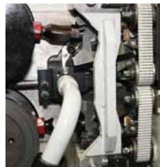
▲ Pinching off the nail point and extraction of cutting waste
