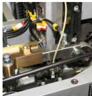
▲ Precise wire feed with mechanically controlled chisel
